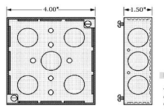
Figure 6-10 Metal 4-in.  $\times$  4-in. device box with a volume of 22.5 in.<sup>3</sup> can contain two switches or duplex receptacles.
