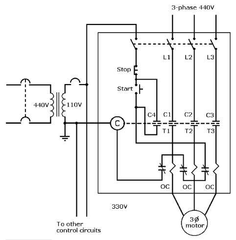
**Figure 10-12** Schematic for an across-the-line motor starter powered by threephase, 440 V AC but controlled by 110 V AC.
