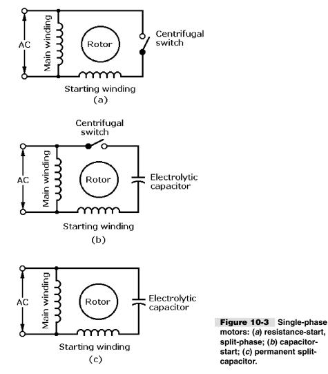
by the centrifugal starting switch when the CS motor reaches about 80 percent of its running speed. The motor then continues to run with only its main winding energized.
