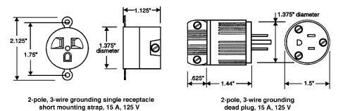
**Figure 6-21** Gallery of outlines and dimensions of straight-blade, locking, and pin-and-sleeve connecting devices.
