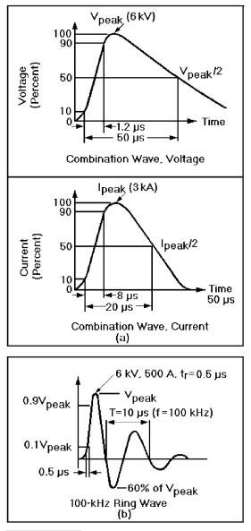
**Figure 12-2** Test waveforms for two types of transient voltage surges defined by ANSI/IEEE C62.41: (*a*) combination wave voltage and current; (*b*) ring-wave transient.
