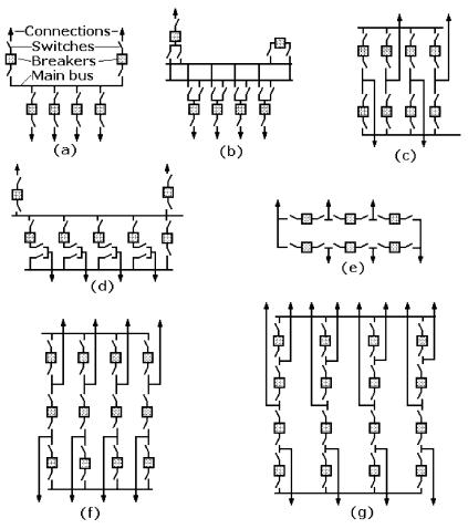
**Figure 4-2** One-line diagrams of substation switching arrangements: (*a*) single bus; (*b*) double bus, single breaker; (*c*) double bus, double breaker; (*d*) main and transfer bus; (*e*) ring bus; (*f*) breaker-and-a-half; (*g*) breaker-and-a-third.
