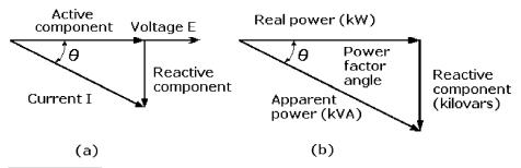
**Figure 3-23** Vector diagrams of active and reactive components in an AC circuit: (*a*) voltage and current; (*b*) real and apparent power.
