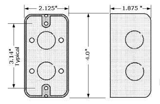
**Figure 6-8** Metal utility 3-in.  $\times$  2-in. device box has a volume of 13.0 in.<sup>3</sup>.
