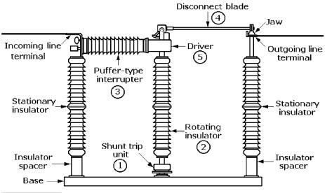
Figure 3-20 Single pole of a blade-type circuit switcher.
