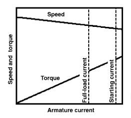
**Figure 10-16** Speed–load and torque–load curves for a shunt motor.
