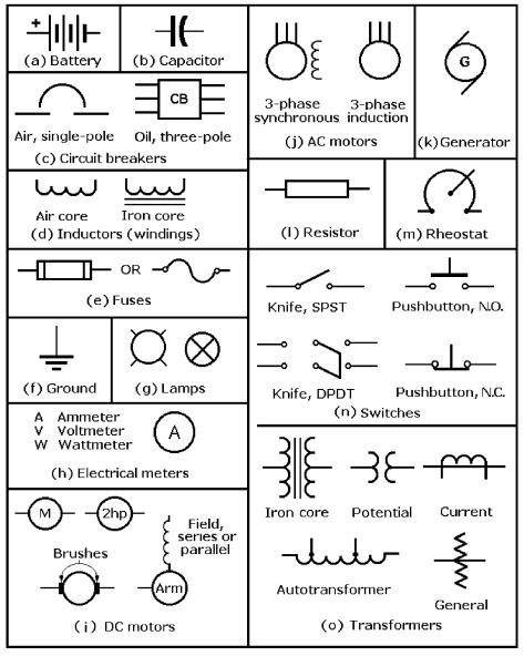
Figure 1-3 Graphic symbols for electrical schematics, Part 1.
