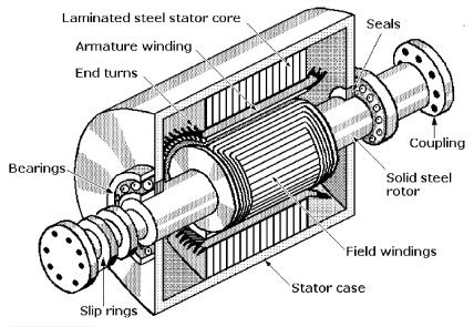
**Figure 2-3** Cutaway view of a synchronous AC generator with a solid cylindrical rotor capable of high-speed rotation.
