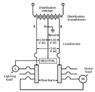
**Figure 5-11** Schematic diagram for a single-phase, threewire loadcenter.
