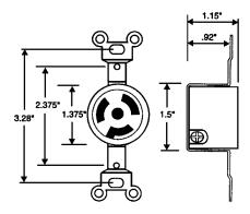
2-pole, 3-wire grounding single receptacle, 15 A, 250 V
