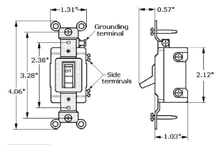
**Figure 6-12** Single-pole AC toggle switch rated for 15 A, 120 V AC has two side and one grounding screw terminals.
