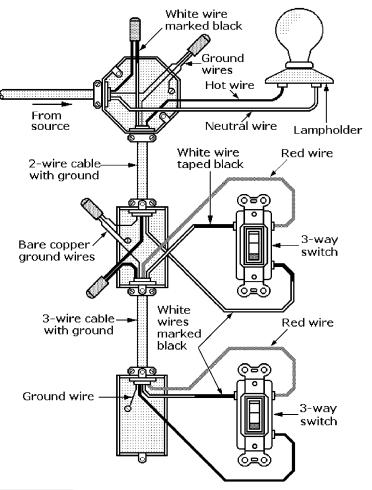
**Figure 7-8** Lampholder at the end of the circuit is wired between a pair of three-way switches.
