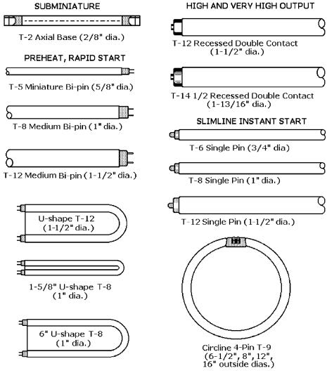
Figure 8-6 Standard fluorescent lamp bulb and base shapes.
