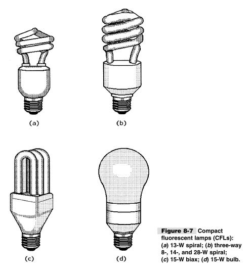
a spiral three-way, an inverted U-shape called bi-ax, and a bulb shape that approximates a conventional A-type bulb shape.
