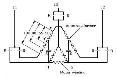
**Figure 10-13** Automatic open-transition autotransformer motor starter.
