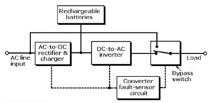
Figure 11-2 Block diagram of an uninterruptible power supply (UPS).
