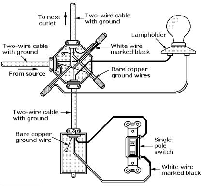
Figure 7-6 Lampholder in the middle of the circuit.
