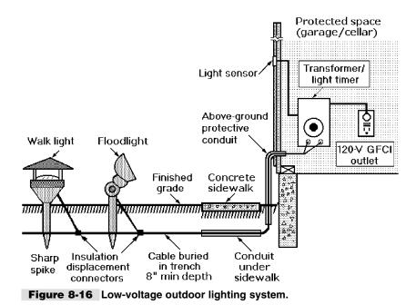
electrical work. The floodlight luminaires include a swivel joint on the mounting stake to permit the lamp to be focused precisely after the supporting stake has been driven into the ground.
