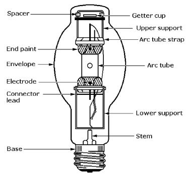
Figure 8-10 Metal-halide (MH) lamp construction.
