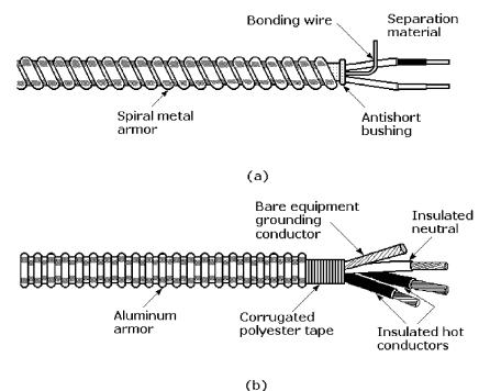
**Figure 6-4** Metal-clad cables: (*a*) flexible armored (AC); (*b*) metal-clad (MC).
