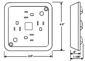
2-pole, 3-wire grounding quad receptacle, 15 A, 120 V
