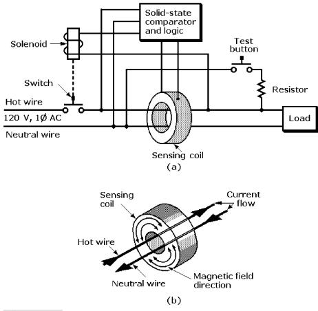
**Figure 6-18** Ground-fault circuit interrupter (GFCI): (*a*) schematic; (*b*) electromagnetic interaction between the wires and sensing coil.
