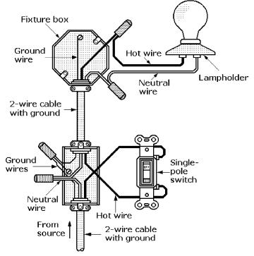
**Figure 7-2** Lamp controlled by a switch: The neutral wire bypasses the switch and goes directly to the lampholder.
