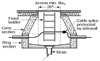
Trap to be installed if drain connects to sewer
