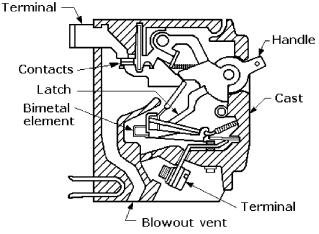
Figure 5-16 Internal view of a thermal circuit breaker.
