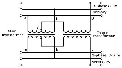
Figure 3-11 T-connected transformers.
