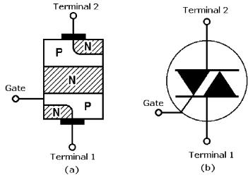
**Figure 3-30** Triac: (*a*) functional diagram; (*b*) schematic symbol.
