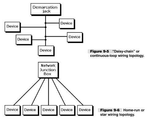
repairs. The flexibility of home-run topology and its elimination of interference and cross-talk between telephones justifies its higher cost, if any, for installation.
