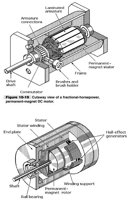
Figure 10-20 Cutaway view of a fractional-horsepower brushless DC motor.
