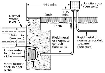
Figure 8-14 NEC-approved installation of an underwater swimming pool lamp.
