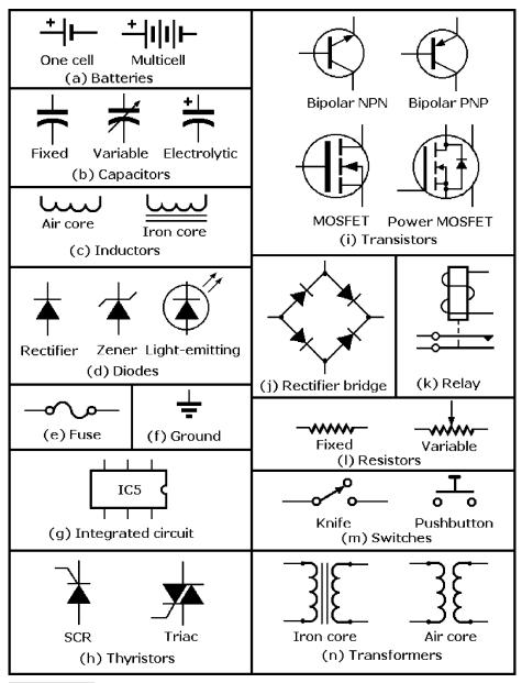
Figure 1-5 Graphic symbols for electronic schematics.
