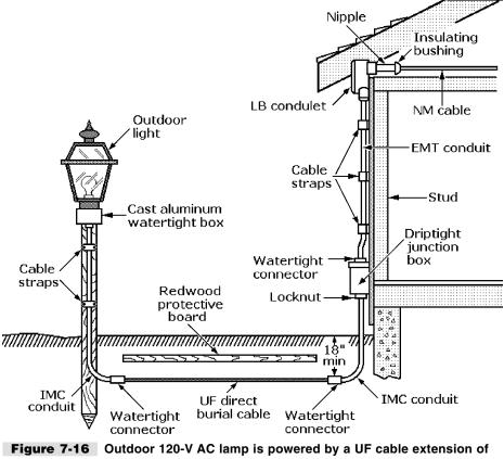
an NM cable from an attic branch circuit.
