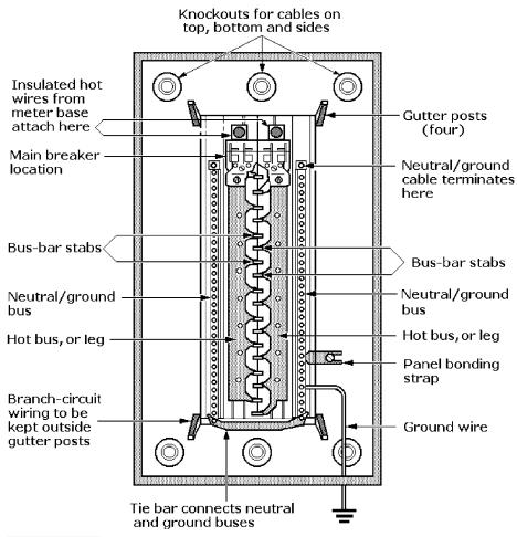
**Figure 5-14** Backpan includes buses for terminating the "hot," neutral, and ground wires, and space for installing circuit breakers and wiring branch-circuit connections.
