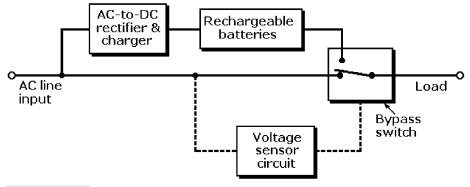
Figure 11-1 Block diagram of a battery-powered standby power supply.
