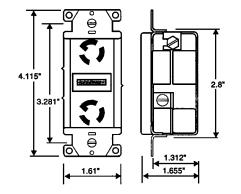
2-pole, 3-wire grounding duplex surge suppressor, 15 A, 125 V
