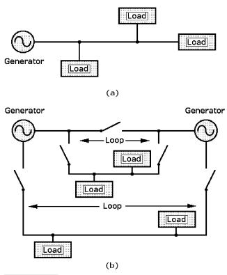
**Figure 4-4** Simplified diagrams of the basic electrical distribution systems: (*a*) radial and (*b*) loop.
