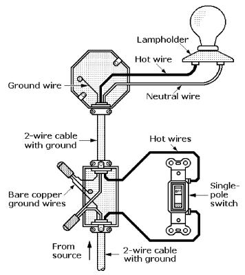
Figure 7-5 Switch in the middle of the circuit.
