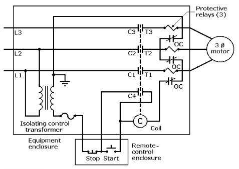
Figure 1-9 Schematic diagram for an across-the-line motor starter.
