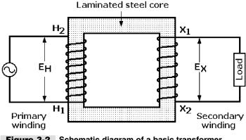
**Figure 3-2** Schematic diagram of a basic transformer.
