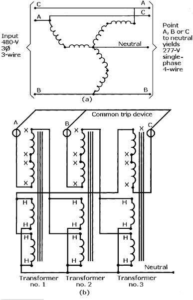
**Figure 3-16** Auto zigzag grounding transformer: (*a*) for deriving a neutral; (*b*) wiring diagram.
