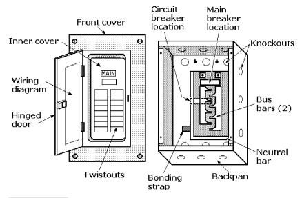
**Figure 5-13** Loadcenter consisting of a front cover with a door and a backpan, where connections are made for incoming and branch wiring to the circuit breakers.
