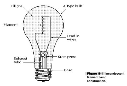
with a glass exhaust tube. The blown glass bulb, which has been coated inside or "frosted," is then sealed to the stem in a machine. Gas flames directed at the mating edges of the glass parts melt them to form a complete envelope.
