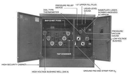
Figure 3-14 Three-phase pad-mounted compartmental-type transformer. Courtesy Cooper Power Systems
