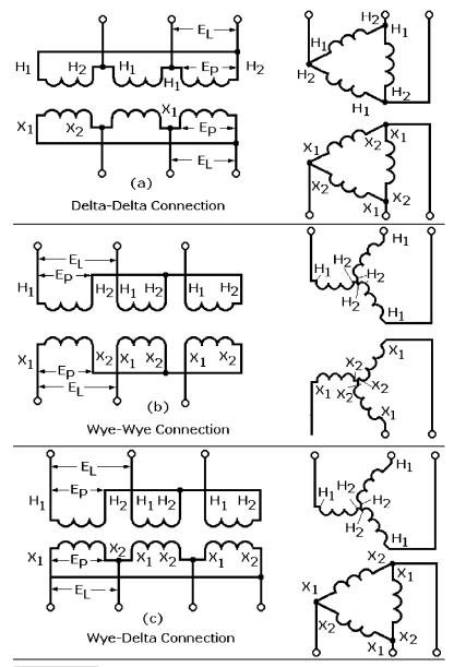
Figure 3-9 Three-phase transformer connections.
