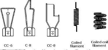
Figure 8-4 Examples of incandescent lamp filament forms.
