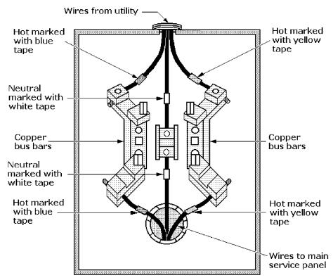
**Figure 5-9** Overhead service to a meter base: color-coded tapes identify wires going into and out of the watthour meter.
