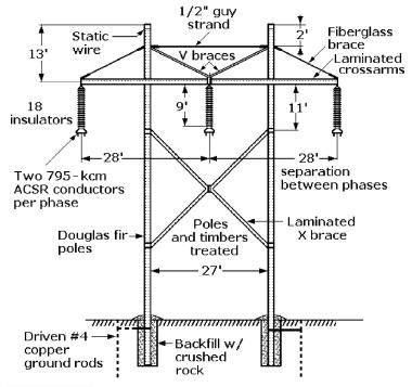
Figure 2-7 A 345-kV wood H-frame transmission tower.
