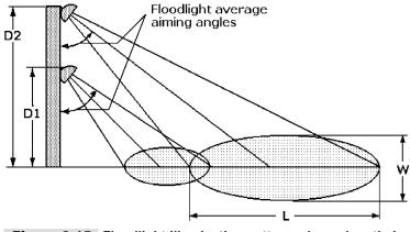
**Figure 8-15** Floodlight illumination patterns depend on their height and aiming angles.
