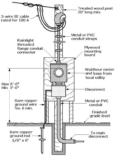
**Figure 5-22** Temporary service entrace assembly rated for 100 A with SE cable exposed to the meter base.
