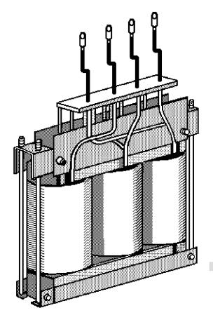
**Figure 3-12** Three-phase core and coil distribution transformer rated for 37.5 kVA, 60 Hz, 2400/4160Y to 240/416Y V.
