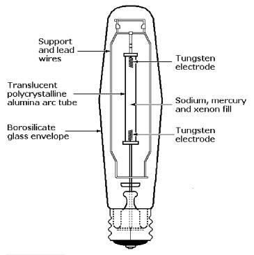
Figure 8-11 High-pressure sodium (HPS) lamp construction.
