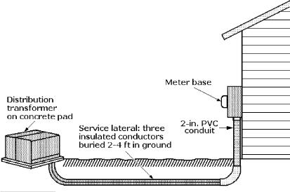
**Figure 5-7** Underground service provides electric power from a padmounted transformer via a service lateral to the service point.
