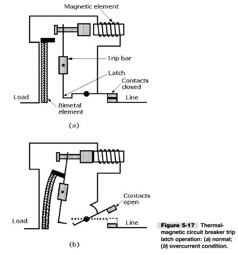
load. If the panel door is left open for a long period of time or is removed, the interior of the panel will cool to a lower temperature. This additional cooling will allow the breaker's thermal element to exceed its rated continuous current. This could mean that the load it is protecting could overheat.
