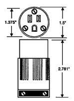
2-pole, 3-wire grounding connectors, 15 A, 125 V
