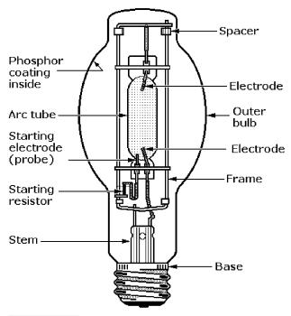
Figure 8-9 Mercury-vapor (MV) lamp construction.
