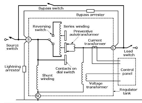
**Figure 3-22** Wiring diagram for a typical distribution step-voltage regulator showing both internal and external connections.
