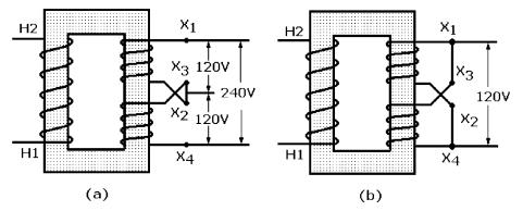
**Figure 3-5** Single-phase transformers: (*a*) connected in series to supply a three-wire, 120/240-V AC system; (*b*) connected in parallel to supply a two-wire, 120-V AC system.
