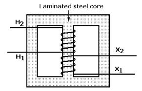
**Figure 3-3** Shell-type transformer core construction.
