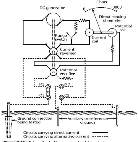
Figure 5-20 Schematic of a Megger ground resistance tester.
