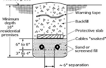
**Figure 4-8** Section view of a trench containing direct-burial cables in nonresidential areas.
