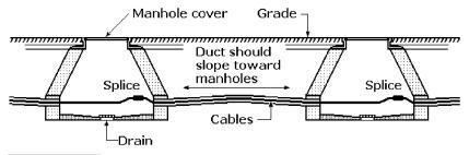
Figure 4-10 Section view of a typical underground duct system.
