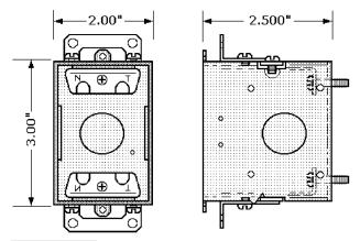
**Figure 6-7** Metal 3-in.  $\times$  2-in. gangable device box sized for a single switch or duplex receptacle has a volume of 12.5 in.<sup>3</sup>.
