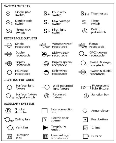
Figure 1-2 Graphic symbols for electrical wiring diagrams.
