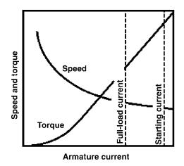
**Figure 10-17** Speed–load and torque–load curves for a series motor.
