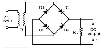
Figure 3-27 Full-wave rectifier circuit contains a bridge of four silicon diodes, a transformer, and an output resistor.
