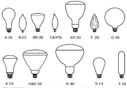
**Figure 8-2** Incandescent lamp bulb shapes: Alphanumerical codes identify the shapes and major diameters in eighths of an inch.
