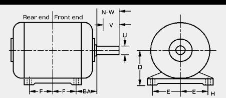
Some key standardized dimensions established by the National Electrical Manufacturers Association (NEMA) are listed below. They apply to all basemounted motors that carry a NEMA frame designation. Letter designations for dimensions not listed are explained in the text. All dimensions are in inches.
